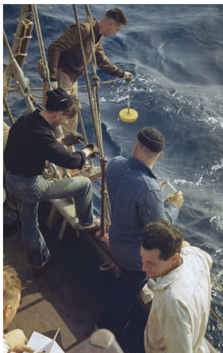
Figure 1 | The simplest of all oceanographic instruments. In this photograph, from 1949, a Secchi disk is being lowered into the sea to measure water transparency.
